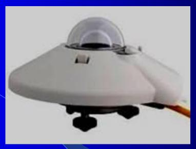
Pyranometers are used to measure the solar radiation. It is a radiometer used to measure all radiation incident on its flat receiver from a 2-pi steradians hemisphere.
