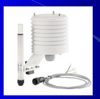
This uses a capacitor which consists of two metal plates separated by a thin polymer film. The film absorbs or exudes water vapour as the humidity increases or decreases, thus changing the dielectric constant of the film. This in turn changes the capacitance of the unit, which can be recorded electronically. The capacitance can then be converted to a measure of humidity using suitable conversion formulae. These instruments are very portable and can be calibrated to quite high accuracy.
