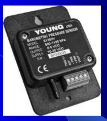
Tiny silicon diaphragms attached to a capacitance gauge which bends to different degrees depending on the external pressure, altering the capacitance of the attached capacitor. Data from these instruments can easily be recorded digitally, allowing high time-resolution studies of pressure-wave events in the atmosphere.
